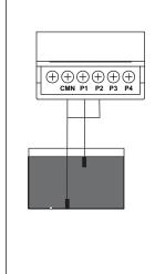
Monitoring 2 Probes): The output relay switches ON which starts up the relay, when liquid level goes above a maximum level, fixed by the probe "P1", When the level drops below a "P1" probe, relay switches "OFF" which stops the relay This operation is not recommended
