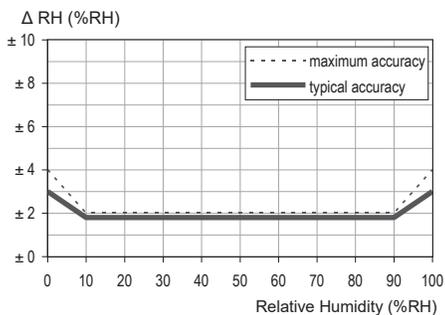
Figure 1. Typical and maximal tolerance at 25°C.
