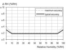
Figure 1. Typical and maximal tolerance at 25°C.
