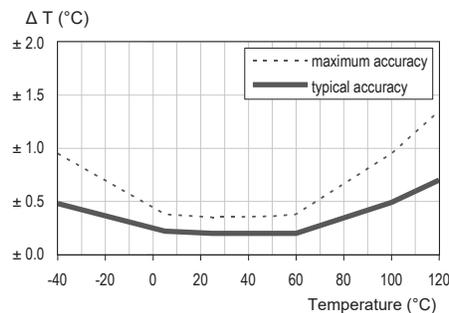
Figure 2. Maximal tolerance for temperature sensor in °C.
